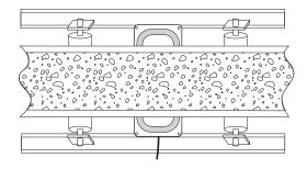
If the coil is installed in a hanging position above the transport belt, always make sure that no structural parts made of iron are too close to the coil and especially that they do not vibrate. If this cannot be avoided, it will be necessary to reduce the sensitivity. This will consequently reduce the detection distance or may have the result that only large pieces of metal will be detected.
