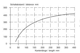
Maximum sensitivity for detector coil MDS 3065 with MDV
