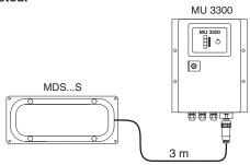
One of the amplifier's tasks is to process the signals emitted by the metal detector coil and convert them into an electronic pulse. The detector coil generates an electromagnetic field. As soon as a piece of metal passes by the coil, it disturbs that field, resulting in a signal that can be evaluated.
