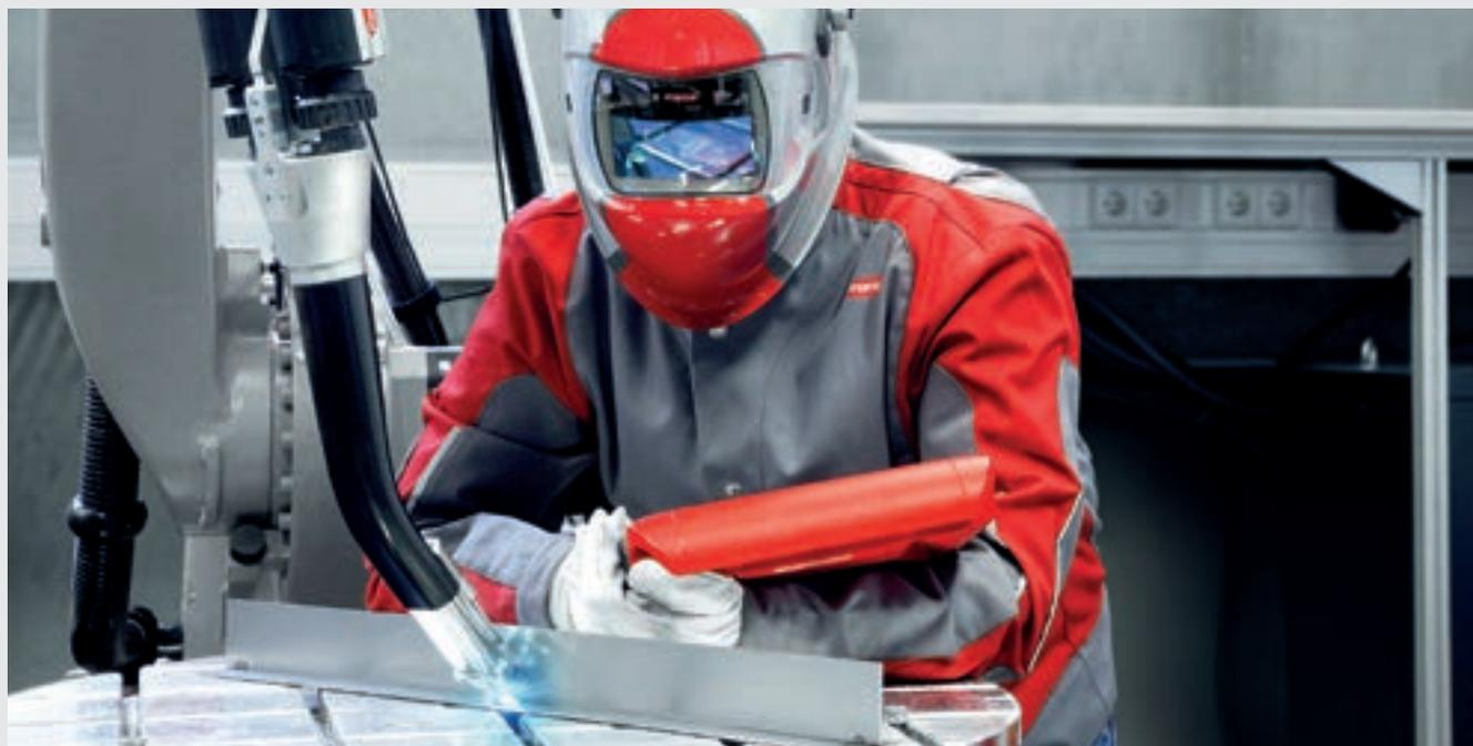
*/ Superior productivity and efficiency with CMT Twin: two power sources, one torch and two insulated contact tips, plus the outstanding welding properties of CMT.*
