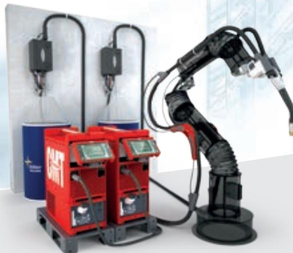
/ CMT Twin is based on the same set-up as the tried-and-tested TimeTwin process: two power sources, one torch and two insulated contact tips ('Lead' and 'Trail'). To which have been added the outstanding welding properties of CMT. CMT Twin scores top marks for its high welding speeds and easy-to-use process control.
