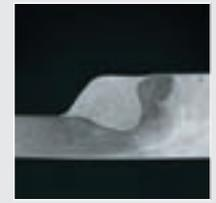
$V_{weld}$  300 cm/min
