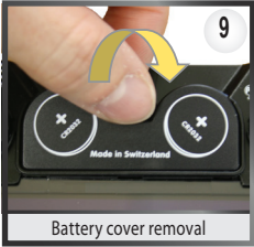
Battery cover removal
