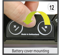
Battery cover mounting
