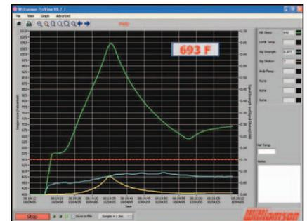
ProView PC software is compatible with Williamson Pro Series sensors. It may be used to log and analyze data and to make remote sensor adjustments.
